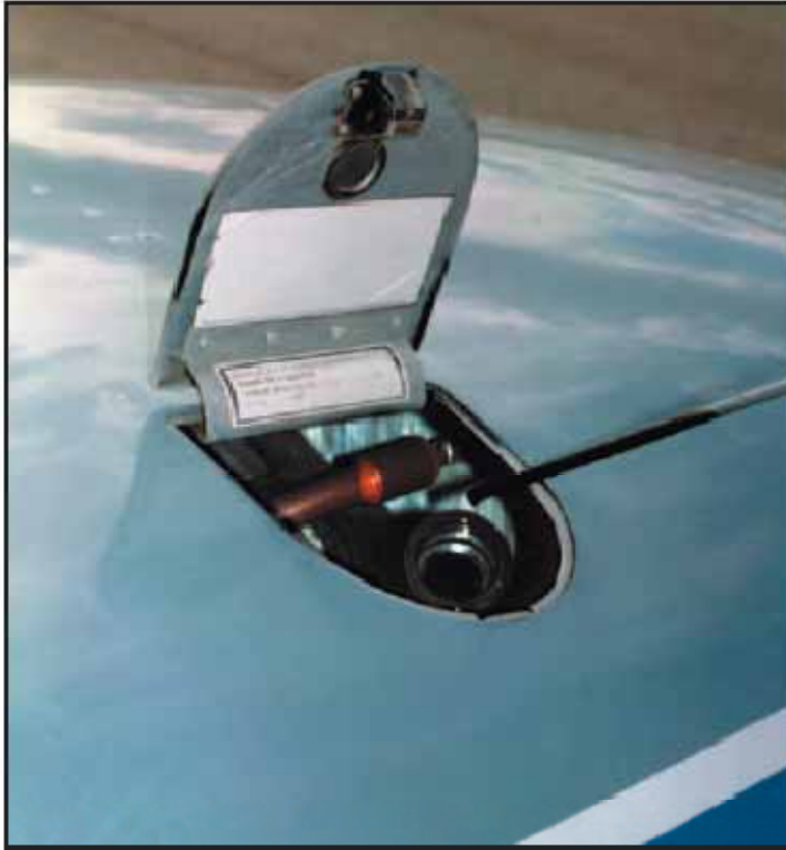
Figure 5-20. Always check the engine oil level during the pre-flight inspection.
