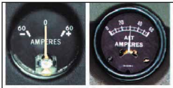
Figure 5-24. Ammeter and loadmeter.
