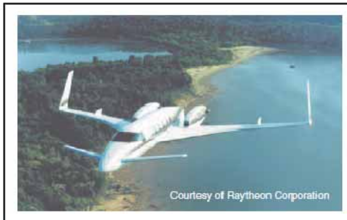
Figure 4-10. This advanced aircraft includes a variable-sweep canard design, which provides longitudinal stability about the lateral axis.
