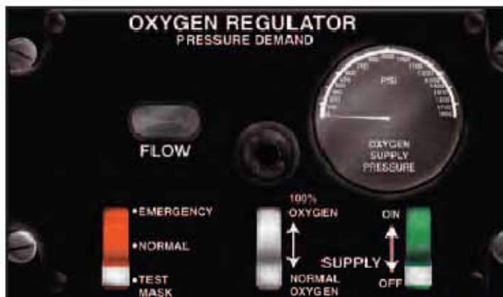
Figure 5-32. Oxygen system regulator.
