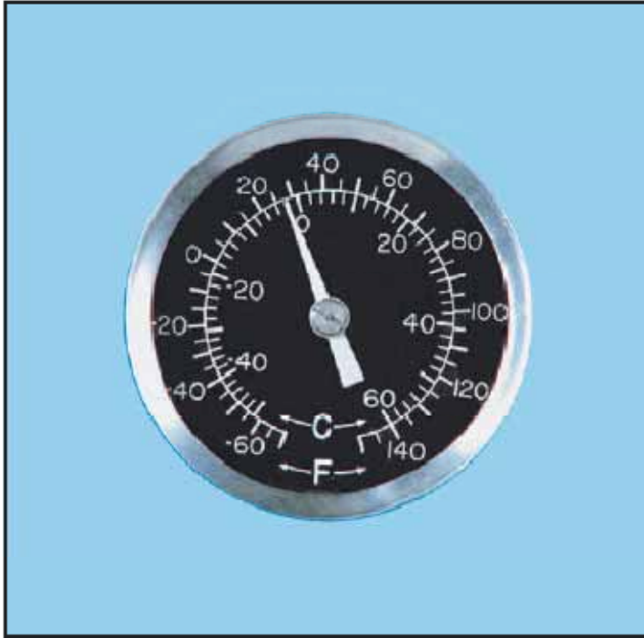
Figure 6-24. Outside air temperature gauge.
